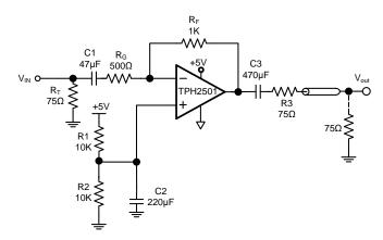
Figure 2. 5V Single Supply Non-Inverting and Inverting Video Line Driver
